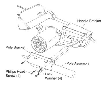
Figure 2 - Attaching Pole Saw Bracket to Handle Bracket
